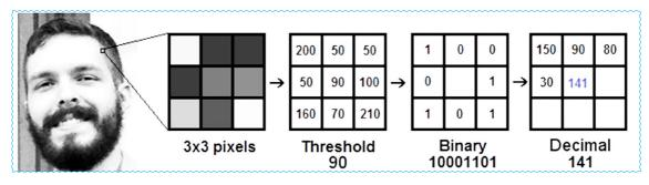
Figure 8: The matrix of the threshold of 3\*3 of LBPH
