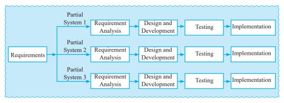
Figure 1: Block Diagram of Incremental Model
